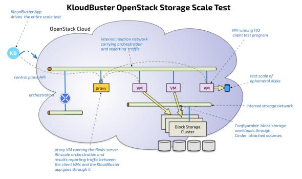
VM staging, storage plumbing (using Cinder or Nova for ephemeral disks) is done by the KloudBuster app using OpenStack APIs. Because the Cinder API abstracts the storage back-end, it is agnostic of the technology used (Ceph, EMC...). After the test, all resources (volumes, VMs, network, router) are cleaned up in the proper order.
