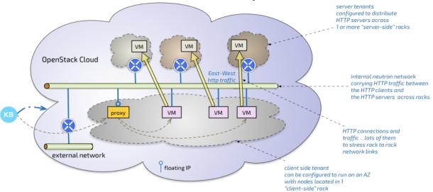
KloudBuster rack to rack East-West dataplane scale test
